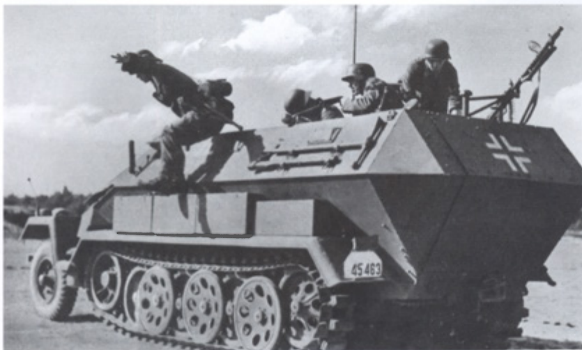
Schützen, or motorized infantry, dismounting from an SdKfz 251/A half-track. Developed in 1937, this innovative vehicle enabled German infantry to keep up with the Panzers and approach the battle area under protection, a concept close to Guderian's heart. (Nik Cornish, WH 312)
